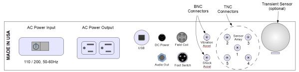
Figure 1 - PIND Controller Back Panel
