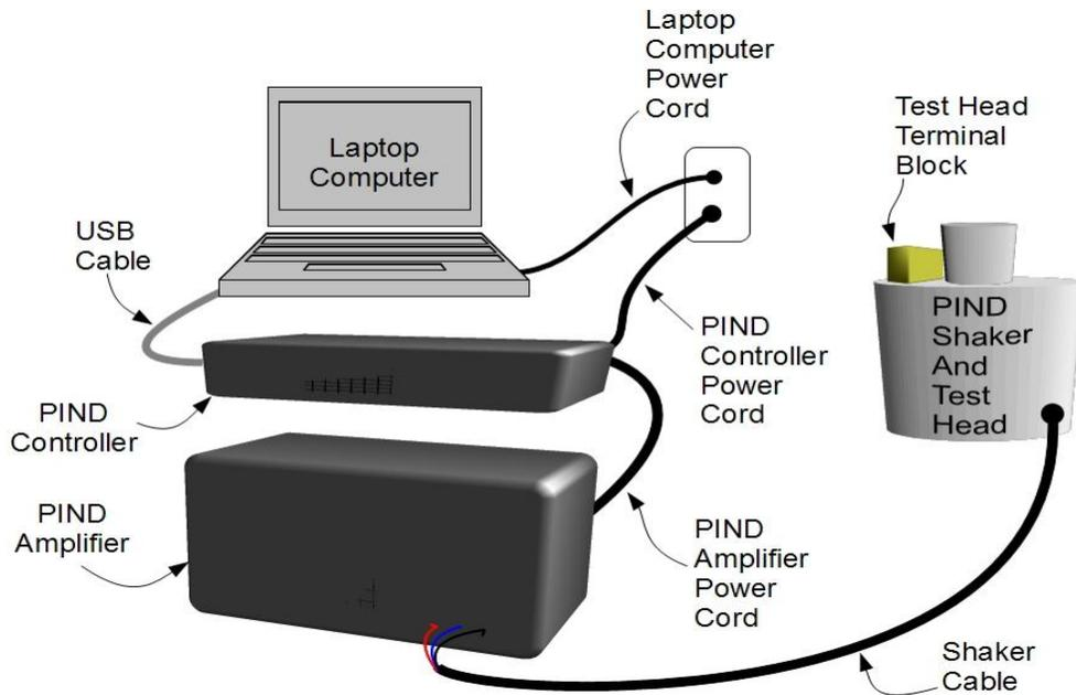
Figure 2 - PIND Test System Components
