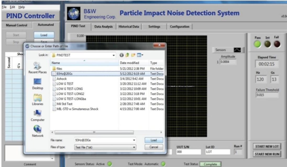
To write a new TEST PROCEDURE follow the diagram below. To change just the frequency it is not necessary to write a new test, just change the frequency and save with new name.
