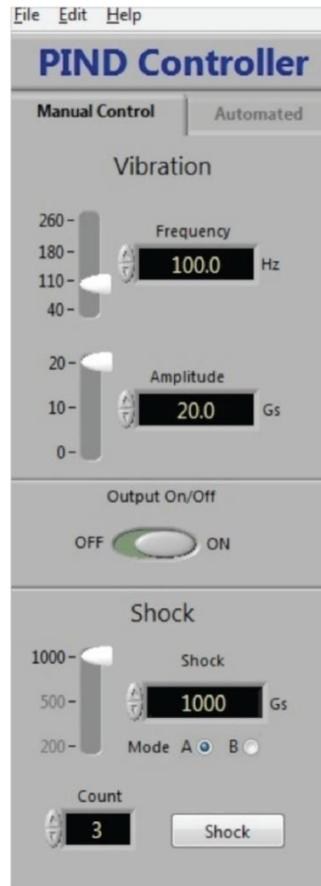
The versatile Manual Mode is useful for experiments and can apply a vibration frequency sweep (to find resonances that make particle type noise) and apply shocks simultaneous with or without vibration. The shock level, count and application can be chosen. In Manual Mode the user has complete control over Vibration frequency and acceleration level and the shock.
