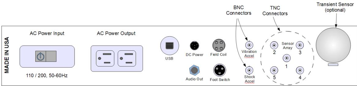
Figure 1 - PIND Controller Back Panel
