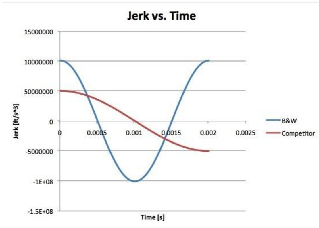
This graph compares Acceleration Change over short time. As the time decreases the Velocity Change over time increases by a factor of 2, 1,000,000 ft/sec<sup>3</sup> @ 50 microseconds vs. 500,000 ft/sec<sup>3</sup> @ 100 microseconds.
